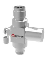
↑ Transmits in the specified frequency range of 0.8GHz to 2.5GHz, behaves as a short circuit during lightning strikes and low-frequency surges, discharging energy to the ground. Widely used for protection in DAS and wireless LAN, typically installed in lightning protection zone LPZO₄-1 and subsequent zones.
