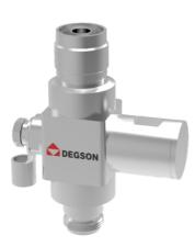
☆ Transmits in the specified frequency range of 0.8GHz to 2.5GHz, behaves as a short circuit during lightning strikes and low-frequency surges, discharging energy to the ground. Widely used for protection in DAS and wireless LAN, typically installed in lightning protection zone LPZO<sub>A</sub>-1 and subsequent zones.
